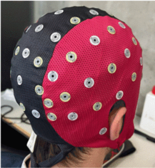
Figure 3.10: CA-204-64 ANT Neuro EEG wet cap, 10-20 system
