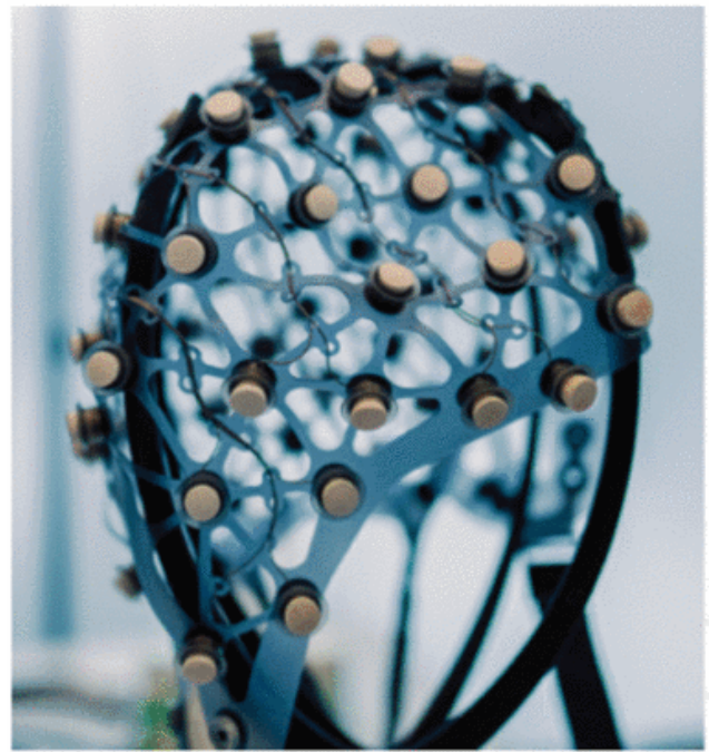
Figure 3.11: NA-261 ANT Neuro EEG semi-dry cap, equidistant system
