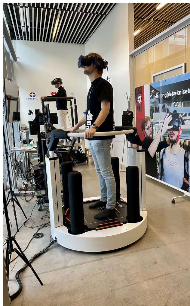
Figure 3.9: New platform with the fixed safety bar
